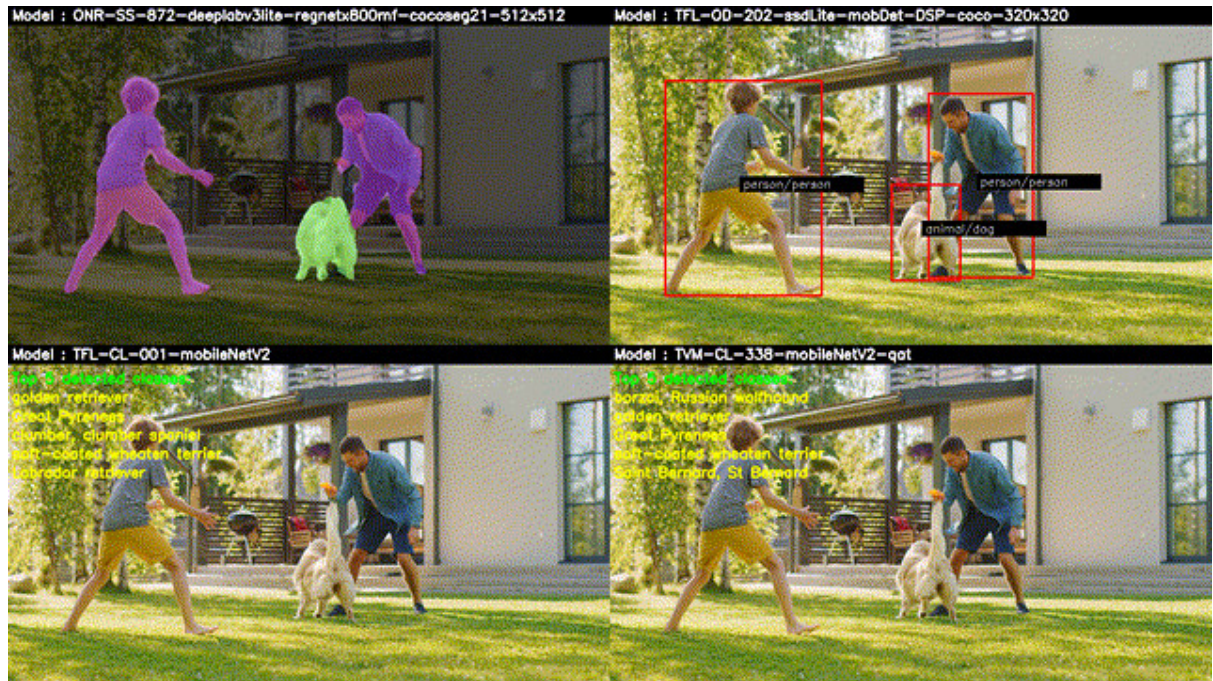
Fig. 5.4: Sample output showing single input, multi-inference output
